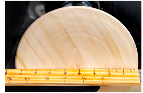
Lay ruler atop tool rest to measure width of green bowl blank.
